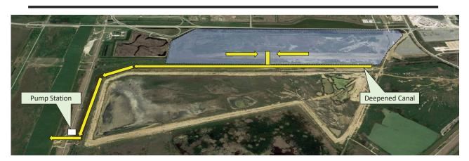
✓ Constructed a single collection point for storm water which is gravity fed to drainage canal
