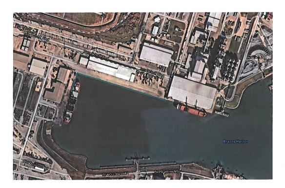
8. Docks 1, 2, 3, 5 and 7 Cathodic Protection – This project involves replacing depleted deep-well anode beds and replacing cabling & boding to the submerged steel structure of the wharfs. The project, once completed, will protect the steel structure from corrosion and deterioration. The budget is \$6,000,000. Contracts have been signed for this project amounting to \$4,026,577. Work has begun.
